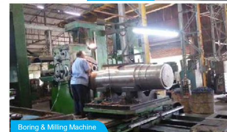
Boring & Milling Machine
