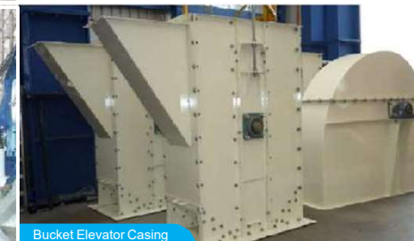
Bucket Elevator Casing
