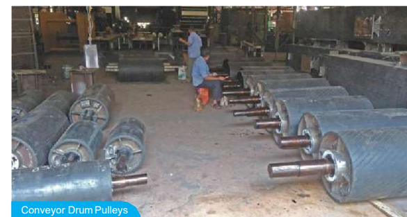
Conveyor Drum Pulleys
